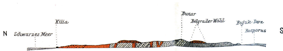
Fig. 8. Cvijić's only coloured cross-section across a part of Istanbul: it goes from the Black Sea coast (Schwarzes Meer) to the Bosphorus. Belgrader Wald is the Belgrad Forest. His legend is: coarse stippling in the north: Diluvial gravels and sands, stippling: alluvium, north dipping lines: quartzite, north-dipping lines with small circles: sandstone and conglomerate, closely spaced, north dipping lines: marls and marly shales, brick symbols: limestones. The cover deposit shown under the Belgrader Wald and one farther to the north are the Belgrad Gravels. Cross-cutting orange rocks with small circles in them are andesite dykes. The cross-section shows that the Thracian-Bithynian erosion surface is older only than the Belgrad Gravels
